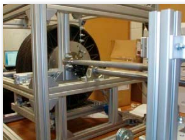
Cryogenic testing equipment developed to test the manufactured lunar wheels. (Image: Dr. Joshua Summers and Clemson University)
